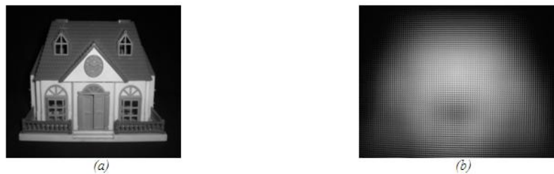
Fig.10 (a) an Image for the Used Home Toy. (b) The Corresponding Elemental Images Array.
